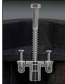
Non-Seizing Bolt System Allows Field Replacement
